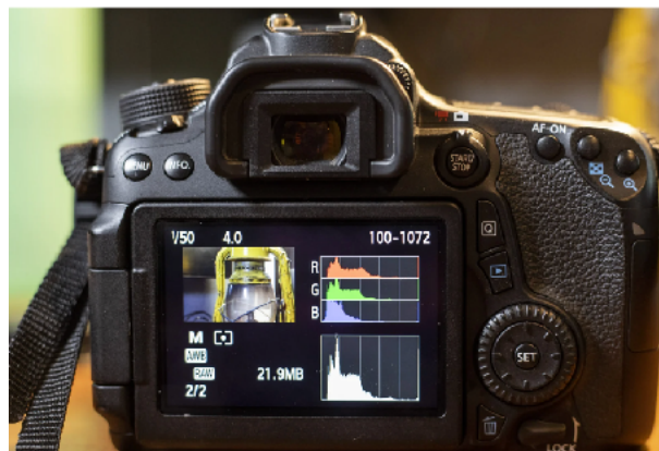
Previewing an image and its histogram on the back of the camera
